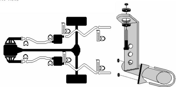
Hanger consists of a metal strap, grommets, hardware and clamp (see illustration).
